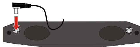
Figure 13 Connect External Power Supply
