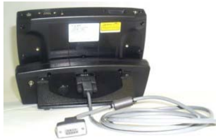
Figure 32 ActiveSync Cable Connected to Serial port on Cradle
