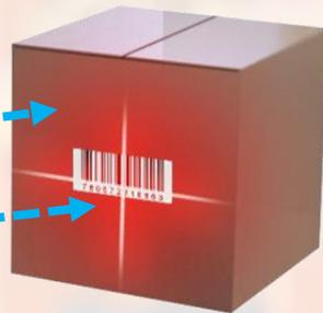
The TC8000 senses that a box has been waved in front of it, using its proximity sensor, and activates the scan engine to decode the barcode.
