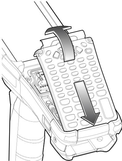
13. Using a Torx T8 screwdriver with a large grip and a long shaft, secure the keypad to the device using the two screws. Torque screws to 5.8 kgf-cm or 5.0 lbf-in.
