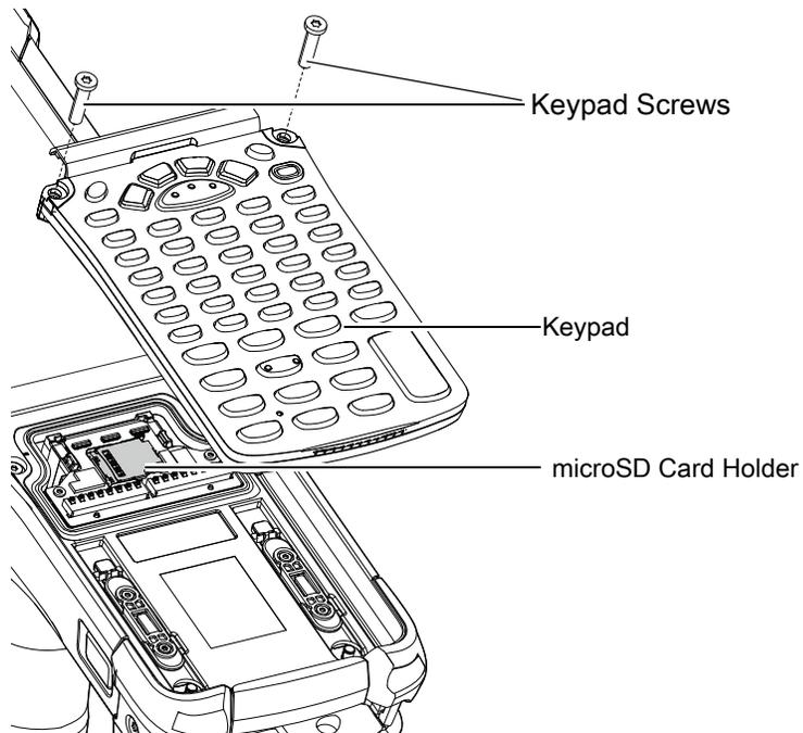
7. Lift the keypad from the device.
