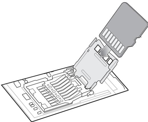
11. Close the microSD card holder door and slide the door to the Lock position.
