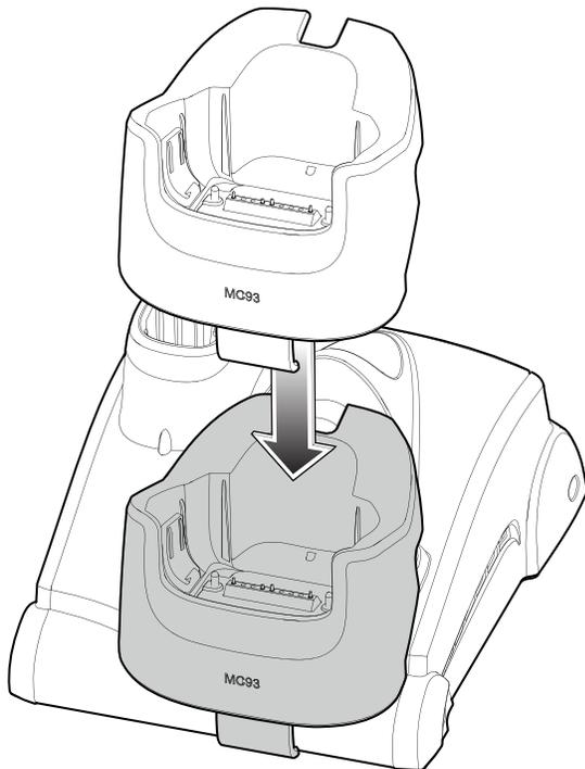
4. Insert the device into the cradle.
