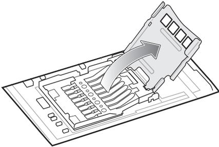
10. Insert the microSD card into the card holder door ensuring that the card slides into the holding tabs on each side of the door.
