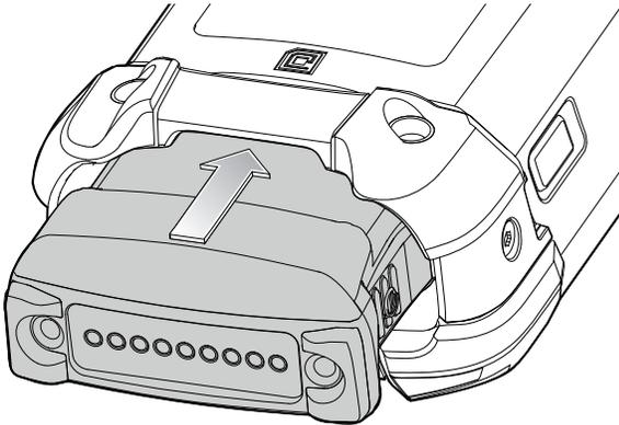
2. Push the battery into the battery slot.
